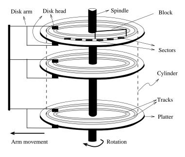
Figure 7.2 Structure of a Disk
